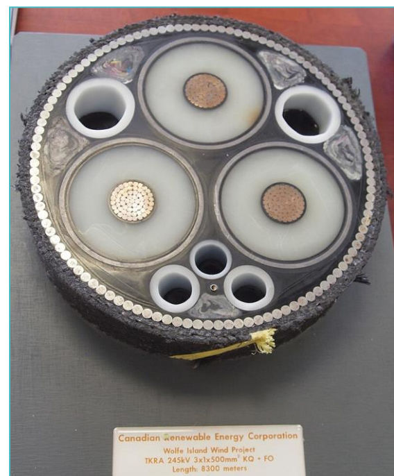
Figure 8: Cross section of a submarine power cable. By Z22.
